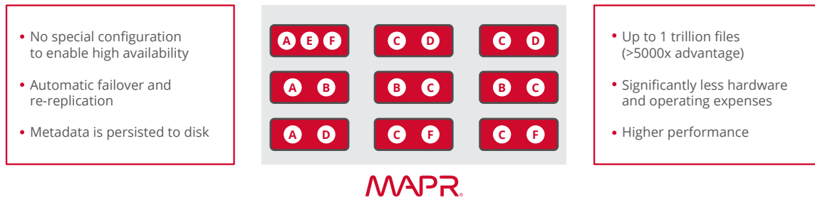
Figure 2: No-NameNode Architecture in the MapR Distribution for Hadoop
